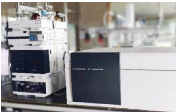
High performance liquid chromatography-mass spectrometry (LC-MS) systems
