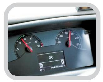
The bus fleet has installed a Speed Limiting Retarder that can automatically activate the brake to prevent speeding downhill
