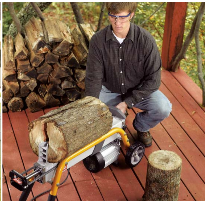
(above) Ryobi Log Splitter, splits logs up to 20" long with 4 Ton of RAM Splitting force.
