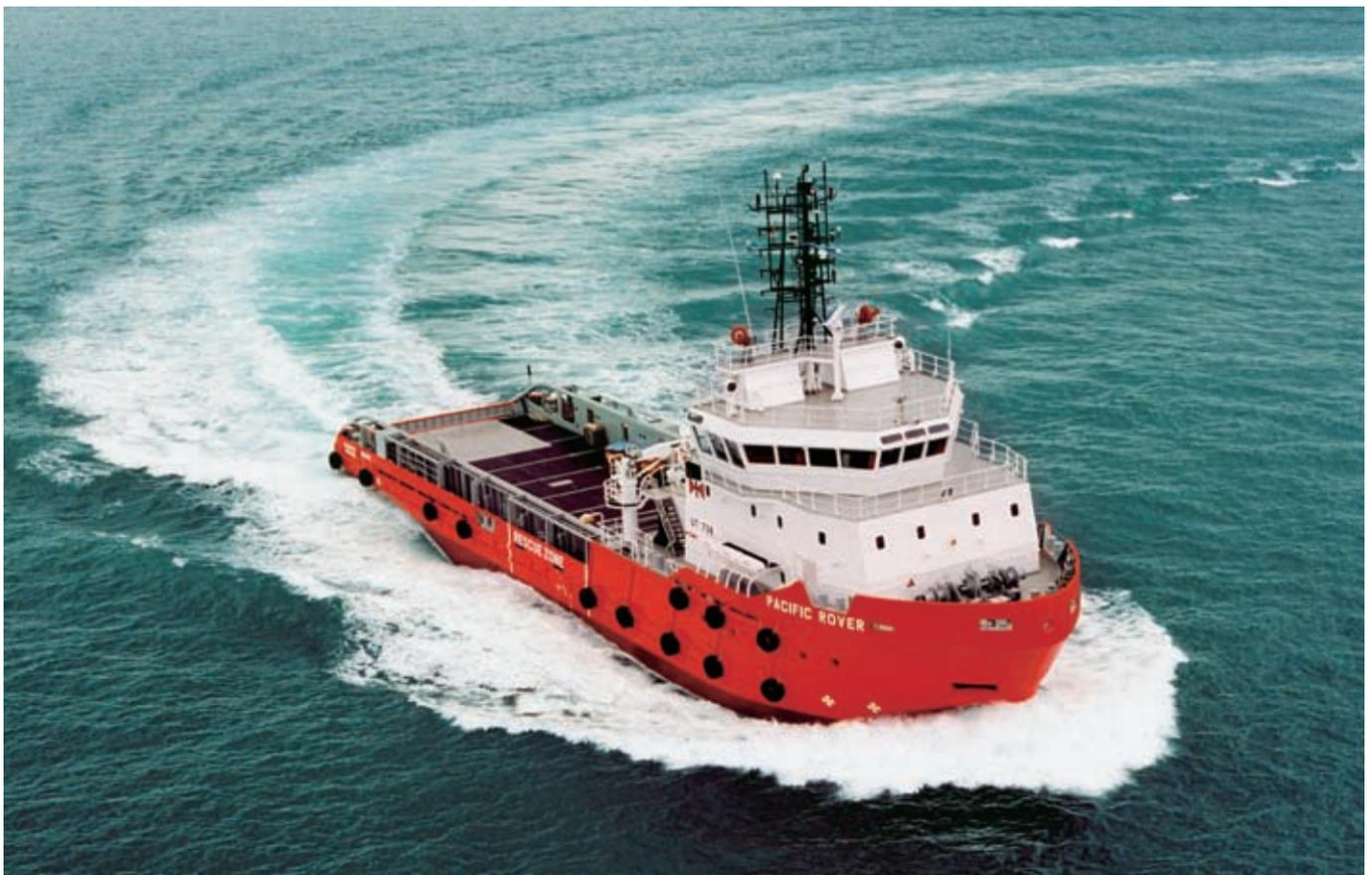
Pacific Rover, an anchor handling tug supply (AHTS) vessel.
