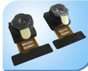
EDOF (extended depth of field) handset camera module
