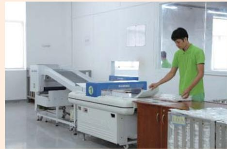
Quality Control — Process of Needle Detection
