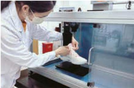
Thermal and moisture permeability test of shoes
