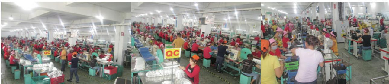
Compared to traditional line processing, the number of workers on a concept line can be significantly reduced. The design of a concept line allows us to improve our quality checks with immediate spotting and correction of errors. While traditional line processing allows us to count for output on certain days of each month, daily output of a concept line is more transparent. The concept line production method certainly enables faster shipment to customers.
