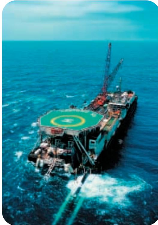
● A barge lays the new pipeline for Hongkong Electric to carry environmentally friendly natural gas from Shenzhen to East Lamma Island for future LNG-powered turbines.
