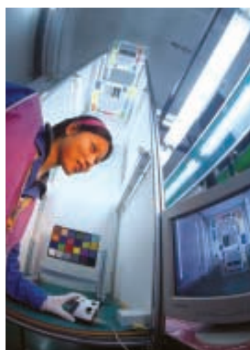
An HHR quality check staff member tests the final assembly of digital cameras to ensure the accurate focusing calibration.
