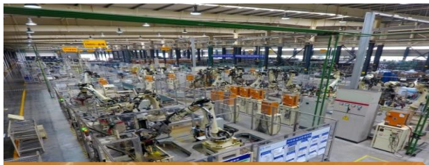
Automated Robotic Welding
