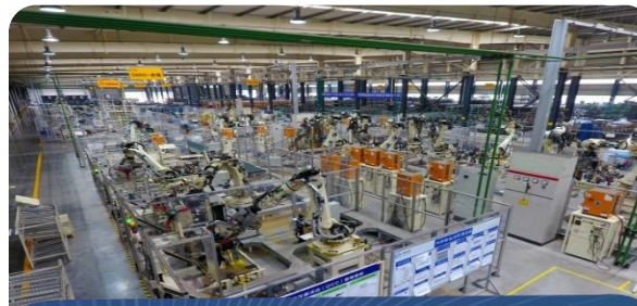
Automated Robotic Welding
