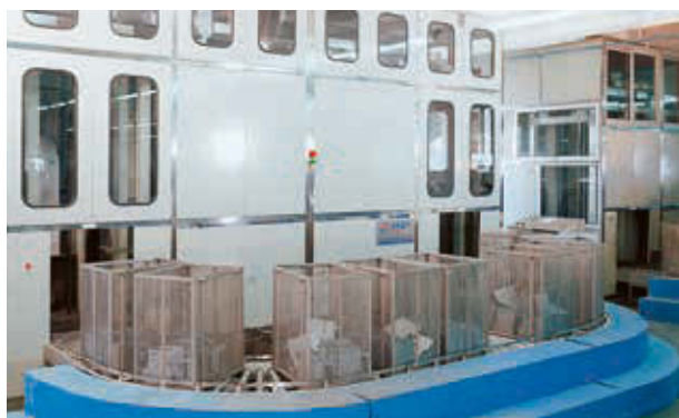
We use ultrasonic cleaners to clean our metal products to replace the traditional method of using corrosive liquids
