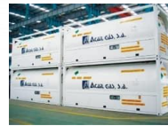
Industrial Gas Tank Container
