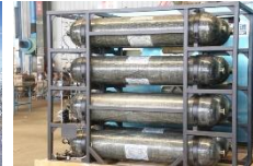
Type III on-vehicle hydrogen cylinders and supply systems
