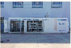
Methanol reforming hydrogen production equipment
