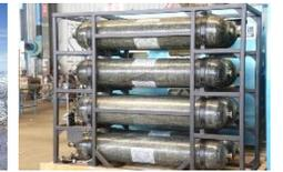
Type III on-vehicle hydrogen cylinders and supply systems
