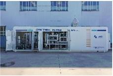
Methanol reforming hydrogen production equipment
