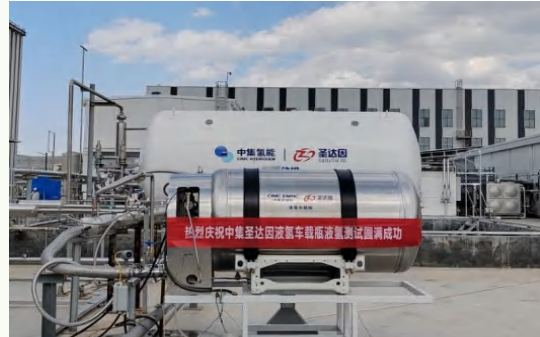
Successful Key Performance Test of Liquid Hydrogen Medium for Vehicle-mounted Liquid Hydrogen Cylinders
