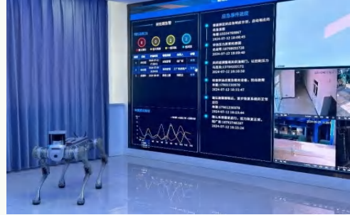
Robotic Dog Inspection and Safety Alert System
