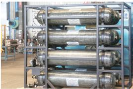
Successfully developed its own 35MPa Type III on-vehicle hydrogen cylinder
