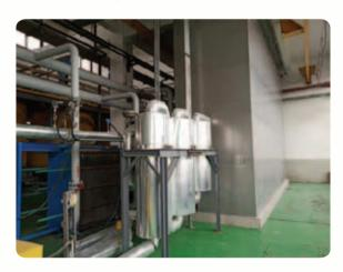
2. Utilising the difference in osmosis of different molecules when passing through VC high pressure nanofiltration membrane, and by separating water molecule from materials, material content is increased while steam consumption is lowered.
