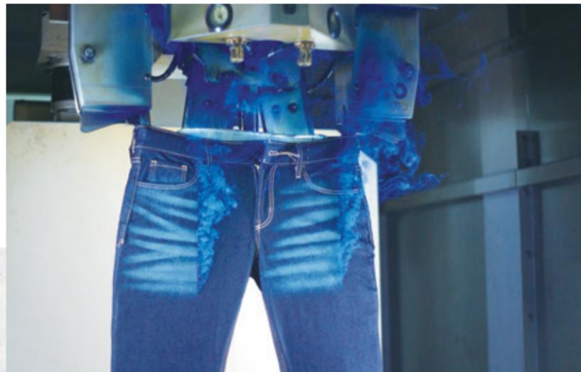
Laser technology — saving five to seven litres of water per garment piece on average — was used in the production of 12.6 million pieces of denim wear in our factories during the year.
