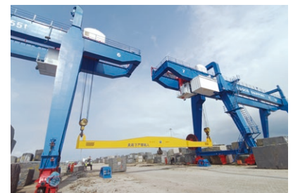
Gantry crane interlocking and twin-lifting
