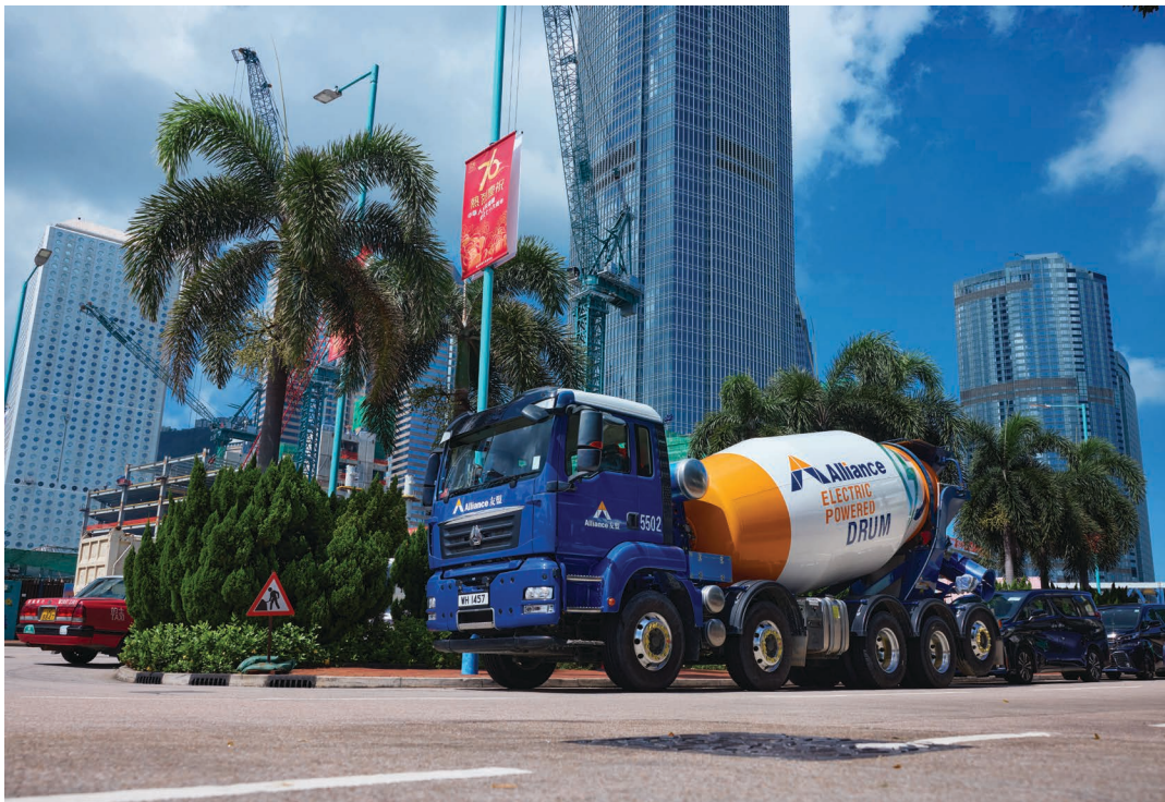
Battery-electric concrete mixer truck at Alliance Construction Materials.
