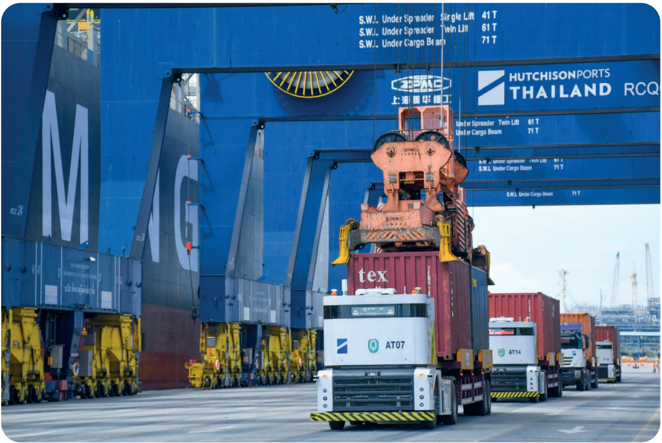
Electric-powered remote-control cranes, Hutchison Ports Thailand
