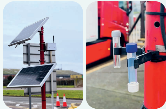
Solar-powered air quality monitoring unit, Hutchison Ports UK
