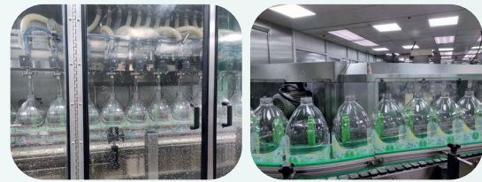
ELF Improvement Project (filling head with volumetric sensor, and bottle washer modification)
