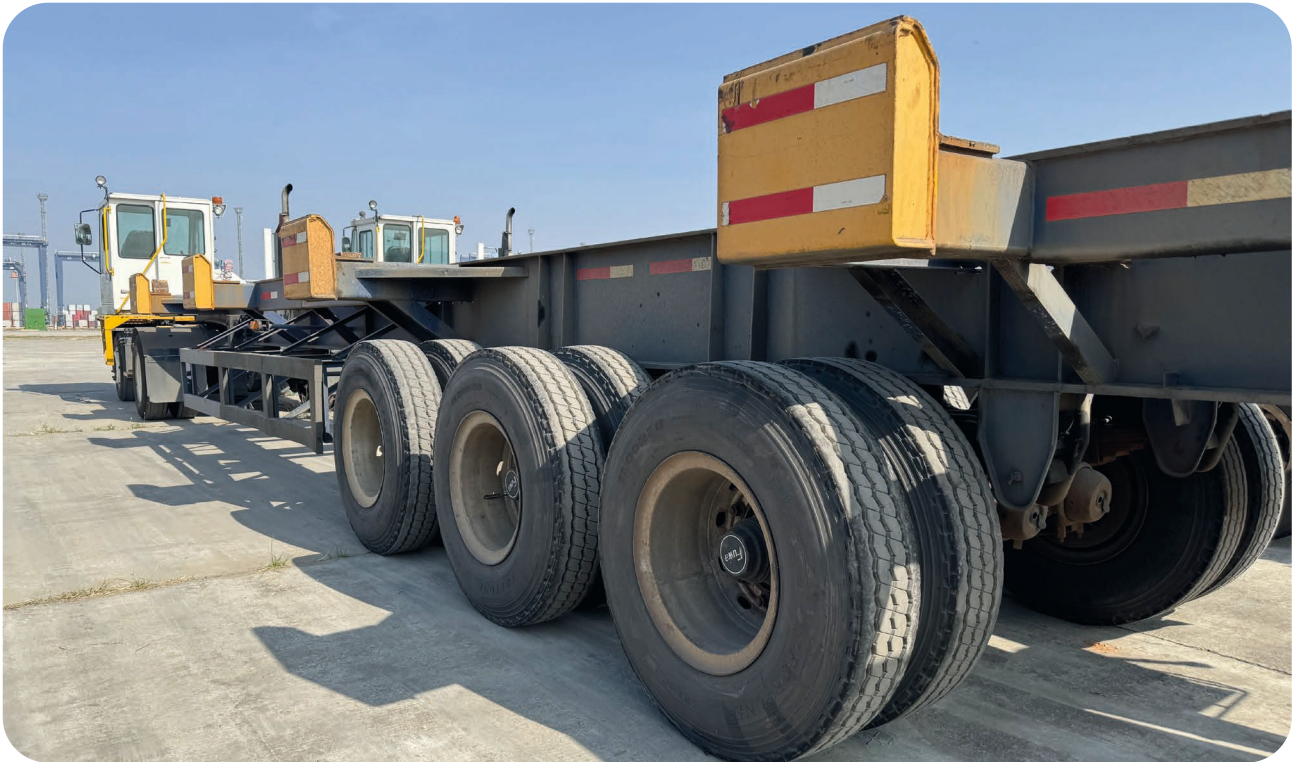
Re-treaded tyres installed at the terminal trailer, Hutchison Ports MITT
