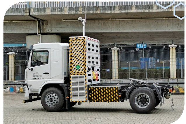
Hydrogen Fuel Cell Trial Tractor at Hutchison Ports Yantian
