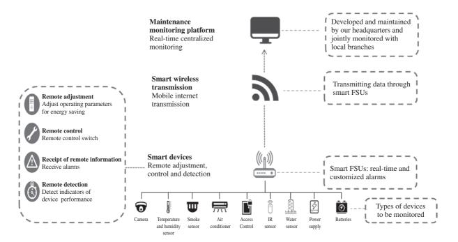
We started compiling the number of monitored sites in April 2016. In 2016 and 2017, there were 1,145,490 and 1,498,577 monitored sites installed with smart FSUs and sensors, respectively. As of December 31, 2017, we had installed smart FSUs and sensors in substantially all sites suitable for remote monitoring. For a small number of sites that cannot be installed with smart FSUs and sensors, we enhance our on-site inspection to ensure smooth operations of our facilities.
