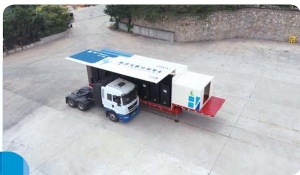
Qiyuanxin Power — charging and battery-swap station for heavy-duty trucks
