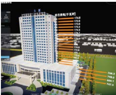
● Green Energy Saving Management – BIM Smart Operation and Maintenance Management Platform
