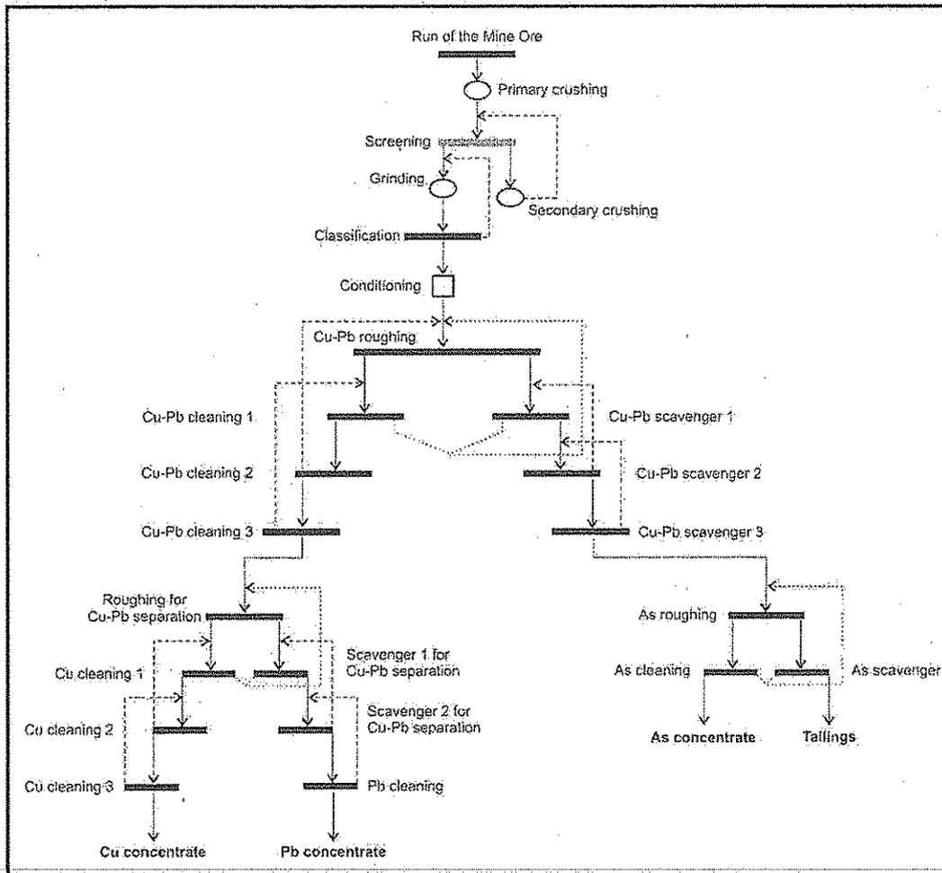
Figure 8.1 Ore Processing Flowsheet for the Damajianshan Mine
