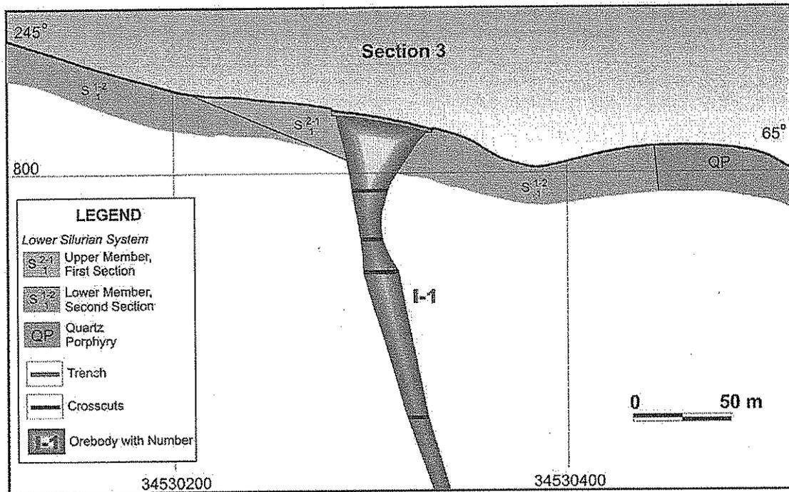
Figure 5.2 A typical Cross Section of the No.1-I Orebody in Damajianshan Deposit
