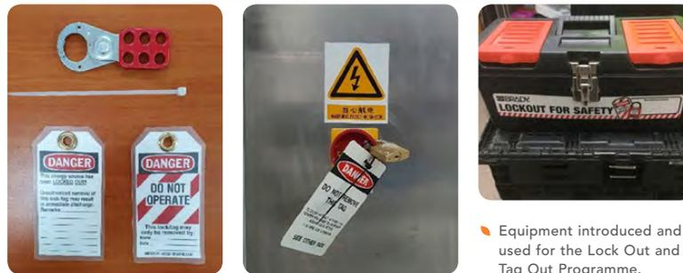
Equipment introduced and used for the Lock Out and Tag Out Programme.
