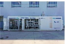
Methanol reforming hydrogen production equipment
