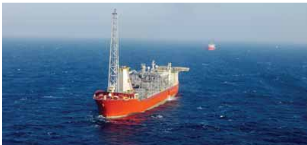
● The SeaRose FPSO (floating production, storage and offloading) vessel produces oil from the white Rose field offshore the Canadian province of Newfoundland and Labrador.
