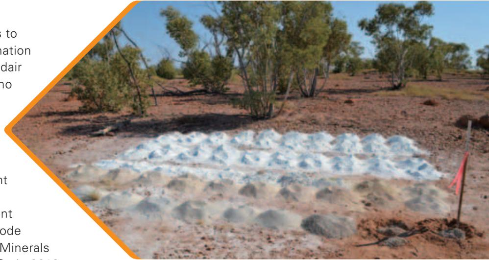
> **Figure 1:** 1m Samples from 70m Rotary Air Blast (RAB) drill hole ready for spear sampling into 4m composites for assay – Lindsay's Lament Prospect
