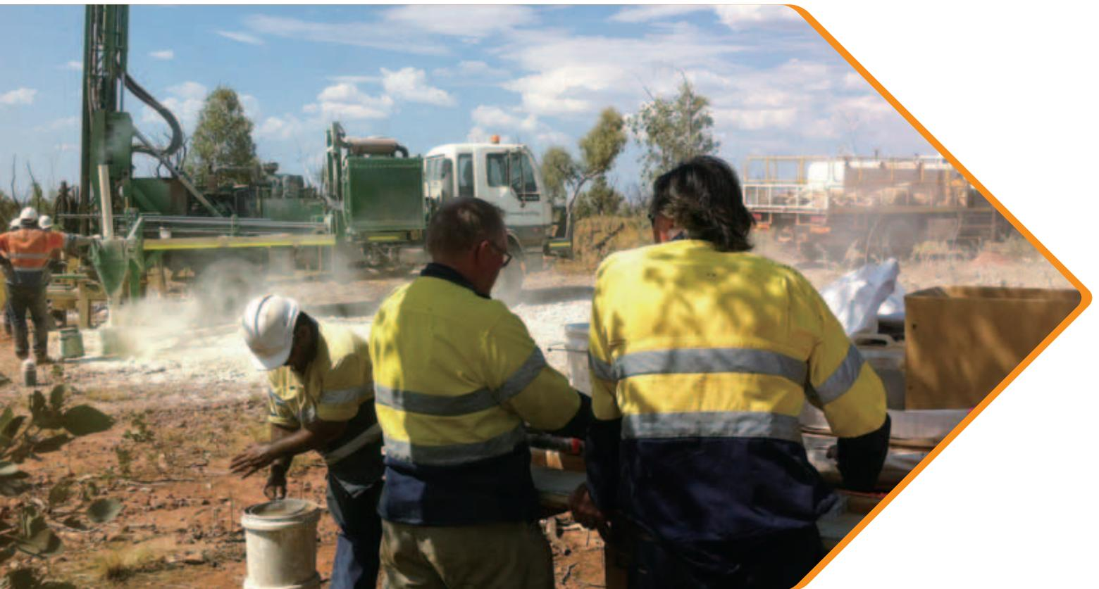
> **Figure 2:** Vertical RAB drilling for oxide copper/lead/zinc mineralisation – CST Western Tenements
