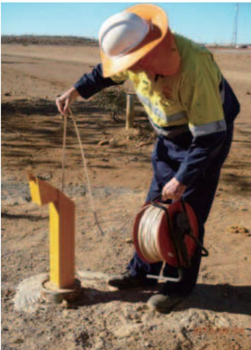
> **Figure 3:** Checking Water Levels in Bore
