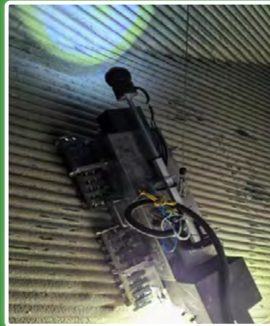
Boiler Water-cooling Wall Inspection Robot
