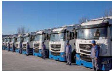
Battery-swapping heavy trucks
